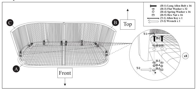
Place Right Arm (B) and Left Arm (C) in corresponding positions on top of Seat Frame (A). Secure with Long Allen Bolts (H-1), Flat Washers (H-3), Spring Washers (H-4) and Hex Nuts (H-5) and stacking the hardware in the order as shown.
