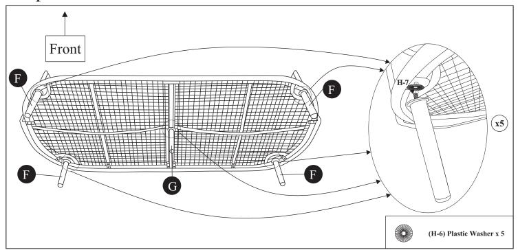
Turn on the assembly on its back onto a clean, non-marring surface. Align bolts on Legs (F), Short Middle Leg (G) and Plastic Washers (H-6) with receiving holes underside as shown. Rotate Legs (F) and Short Middle Leg (G) clockwise until snug. DO NOT OVER TIGHTEN.
