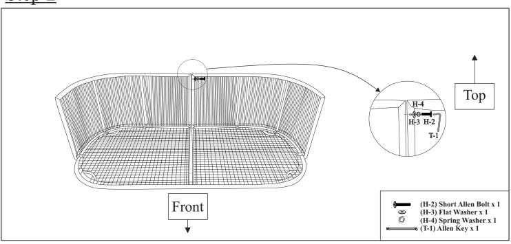
Connect Right Arm (B) and Left Arm (C) with Short Allen Bolts (H-2), Spring Washers (H-4) and Flat Washers (H-3) and stacking the hardware in the order as shown. Engage all hardware by hand, then tighten them using the Allen Key (T-1). DO NOT OVER TIGHTEN.
